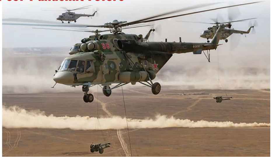
Russian Airborne Troops (VDV) operated Mi-8 utility helicopters to carry D-30 122 mm towed howitzers during the Kavkaz 2020 Military Exercise held in September. Credit: Russian MoD.
